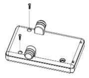
Turnunitover, tiltup slightly, and remove screws at the front of the unit.
