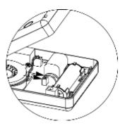
4. Disconnect the leads of the Bulb Assembly from the main circuit board.
