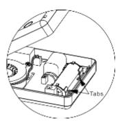
Lift the small circuit board holding the target screen and bulb (Bulb Assembly) from the two tabs.
