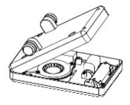
2. With the front remaining tilted up, slide the lower half of the case back and up until it is free.
